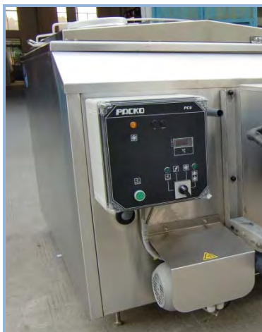
External ice water pump mounted on the tank
