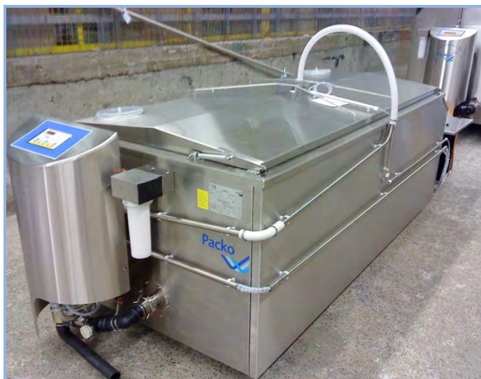
OM/IB milk cooling tank with automatic cleaning
