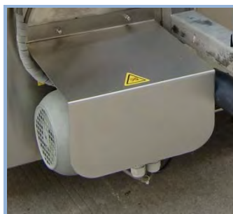
Stainless steel hood protects the ice water pump
