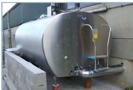
Example of an outdoors REM/DX milk cooling tank – control unit inside the dairy
