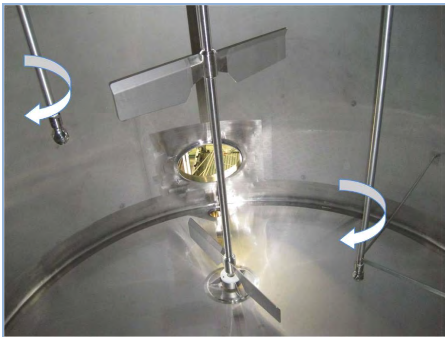
Rotating spray balls on different levels
