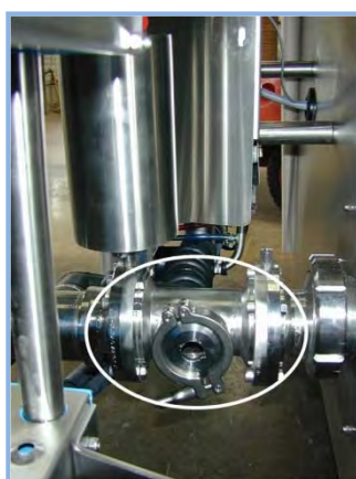
Example of a bottom inlet connection for 1 supply line
