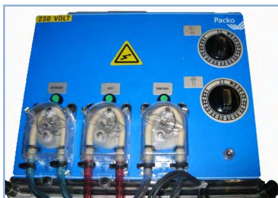
Example of 3 dosing pumps built on the control box
