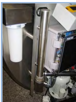
Heating element mounted in line
