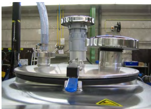
Manhole cover with vent, agitator motor, connection for spray ball
