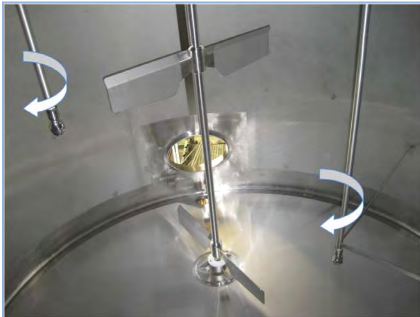
Double agitator paddle and two spray balls at different level
