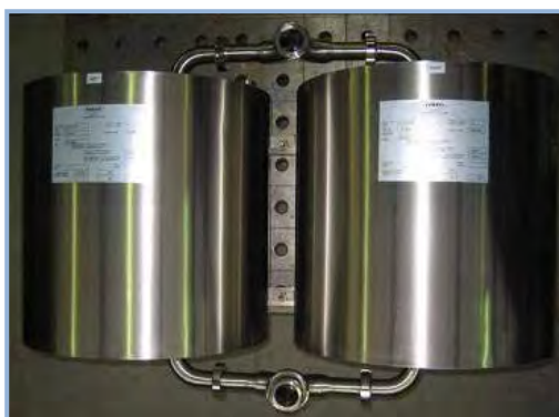
Example of 2 tubular coolers on frame
