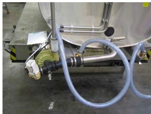
Hoses for in- and outlet ice water Outlet combination with cleaning pump
