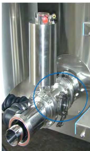
Example of a bottom inlet connection for 1 supply line
